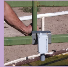
LoRa-enabled DecentLab™ real-time water level sensor
