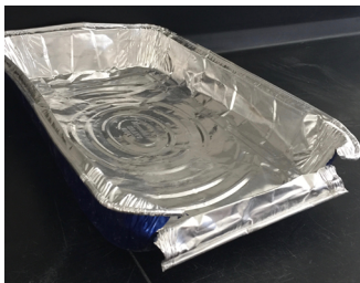
Figure 3. Soil pan, showing cut flap
