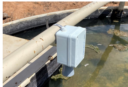
Ultrasonic water level sensor mounted on stock tank
