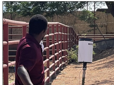
Real time data tipping bucket rain gauge installed near a holding pen.
