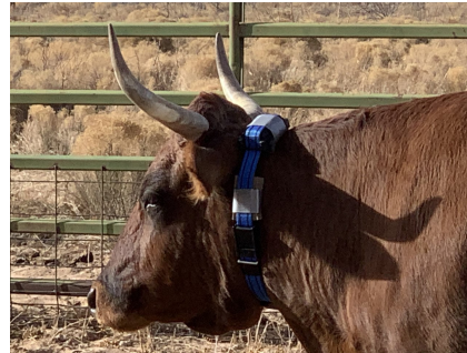
GPS tracking collar worn by a Raramuri Criollo cow.
