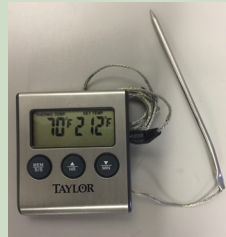
Figure 2. Example meat thermometer with probe and digital readout
