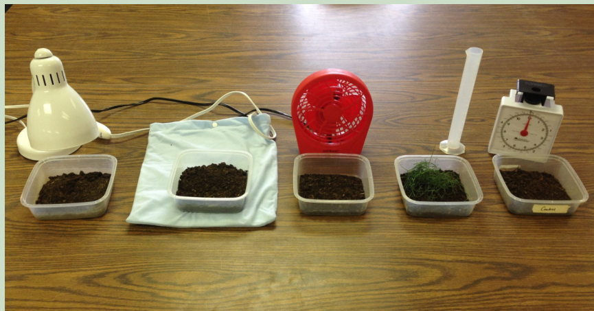
Figure 2. Five experimental containers with treatment materials (left to right): heat lamp, heating pad, desktop fan, Spanish moss, and control
