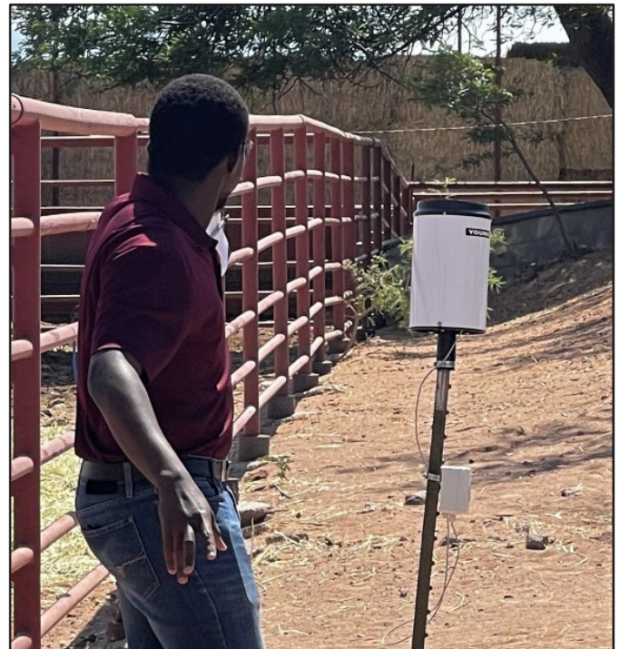
Real time data tipping bucket rain gauge installed near a holding pen.
