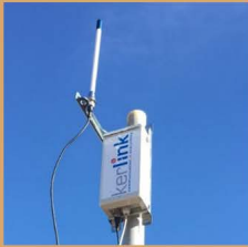
LoRa WAN antenna and gateway
