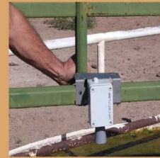
LoRa-enabled DecentLab™ real-time water level sensor
