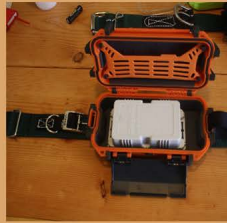
Abeeway™ LoRa-enabled GPS tracker in Pelican water-tight box
